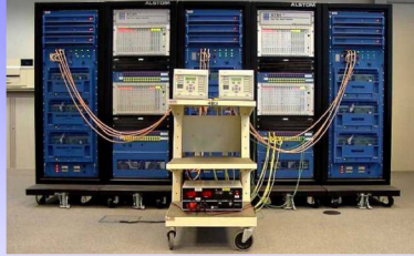
Traditional Closed Loop Relay Test Set-Up
