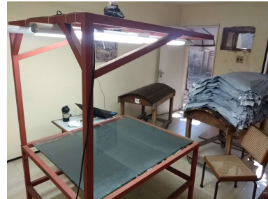
Fig. 1. Table for digitizing leather samples.
