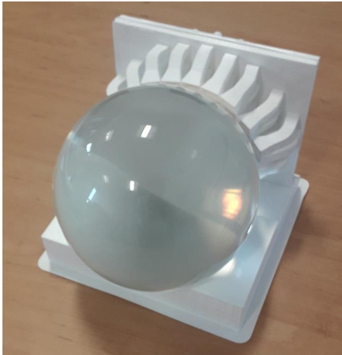
51 beam mmWave beamformer
