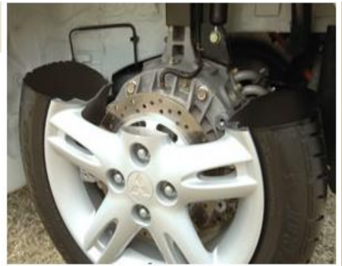
In-wheel motor (on Colt EV)
