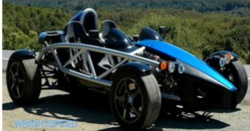
Two seat 1600 lb sports car by Ian Wright in an Ariel Atom chassis Acceleration, 0 – 60 in 2.9 sec, ¼ mile in 11.5 sec, 236 HP, 3 Phase AC Induction motor and drive by AC Propulsion, batteries A123 Systems
