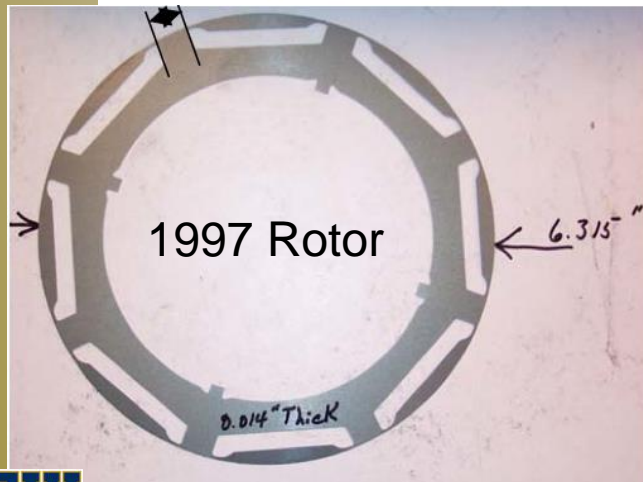
Fig. 2.70. Comparison of motor rotor lamination dimensions.
