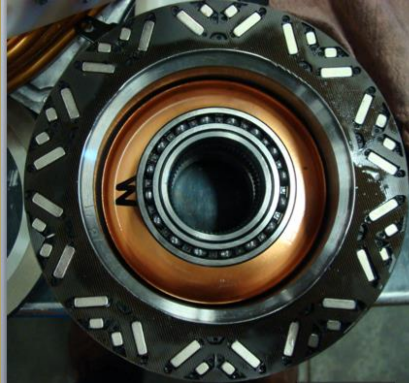
Ten pole IPM, dual layer V
