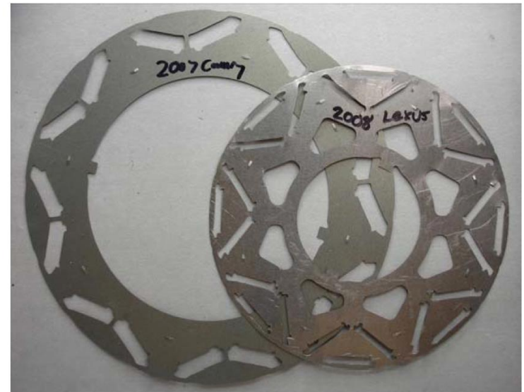
Fig. 2.69. Comparison of motor rotor laminations, Camry (left) vs. LS 600h (right).
