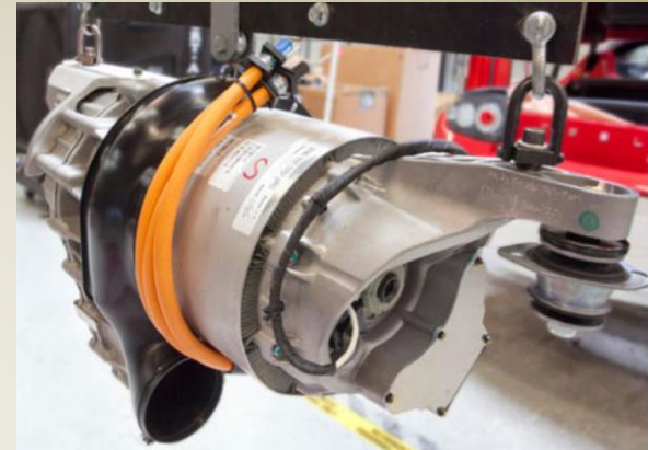
4 Pole AC Induction motors
