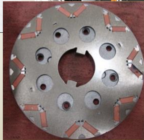
(8) Pole IPM Rotor
