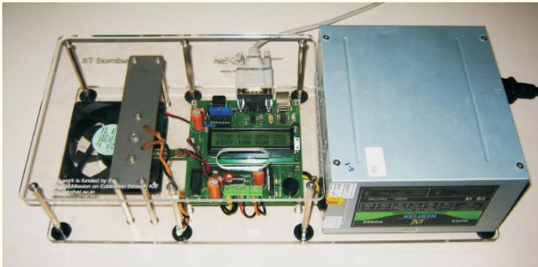
Figure 1: Single Board Heater System
