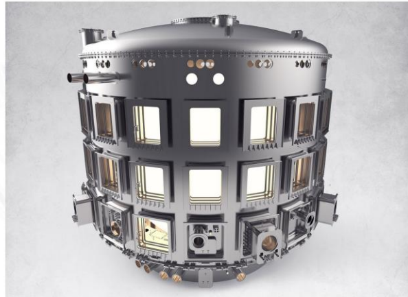
Vacuum Cryostat containing the Tokamak
