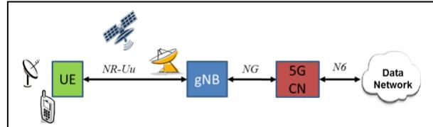
Figure 2: NTN integration based on satellite transparent payload.
