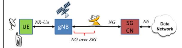
Figure 3: NTN integration based on satellite regenerative payload
