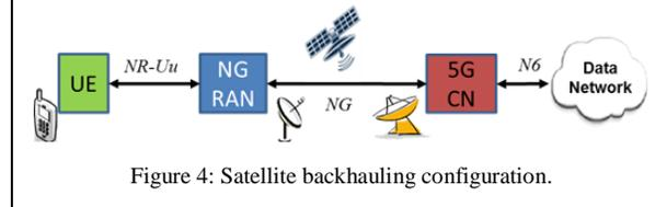
Figure 4: Satellite backhauling configuration.
