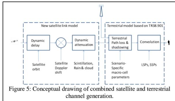
Figure 5: Conceptual drawing of combined satellite and terrestrial channel generation.
