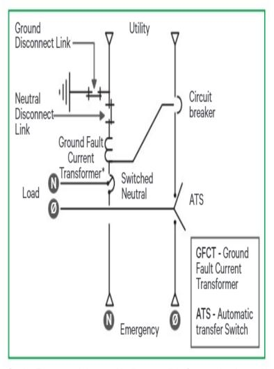
Service Entrance switches provide disconnect links for ground and neutral conductors.\*Ground fault trip protection provided on models of 1000 amps and above
