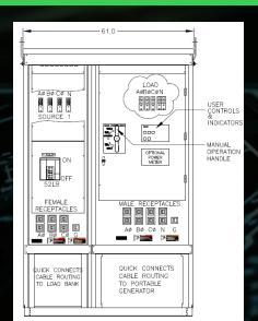
MTDQ – Dual Purpose Manual Transfer Switch with Quick Connects
