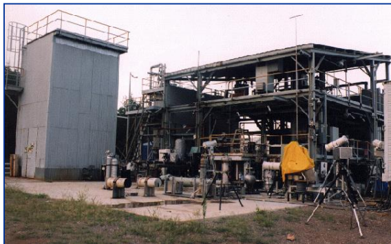
Test Stand 115 7.5 Klbf Thrust Ambient LOX/LH2/CH4/RP
