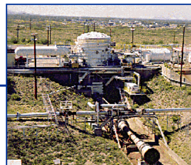
Test Stand 401 25 Klbf Thrust 120 Kft Altitude LH2/LOX/CH4/RP N2O4/Hydrazines
