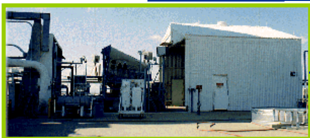
Test Stand 328 25 Klbf Thrust Ambient N2O4/Hydrazines
