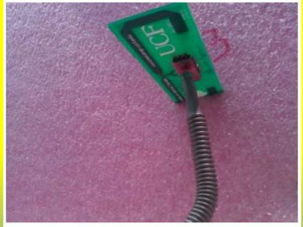
Gas flow test fixture applying H 2 gas
