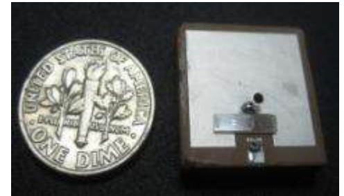
Miniature 915MHz Integrated OFC SAW-Patch Antenna OFC=Orthogonal Frequency Coded SAW=Surface Acoustic Wave
