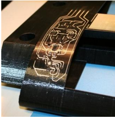
UAV wing with strain sensor
