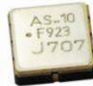
Packaged temperature sensor TSE AS10
