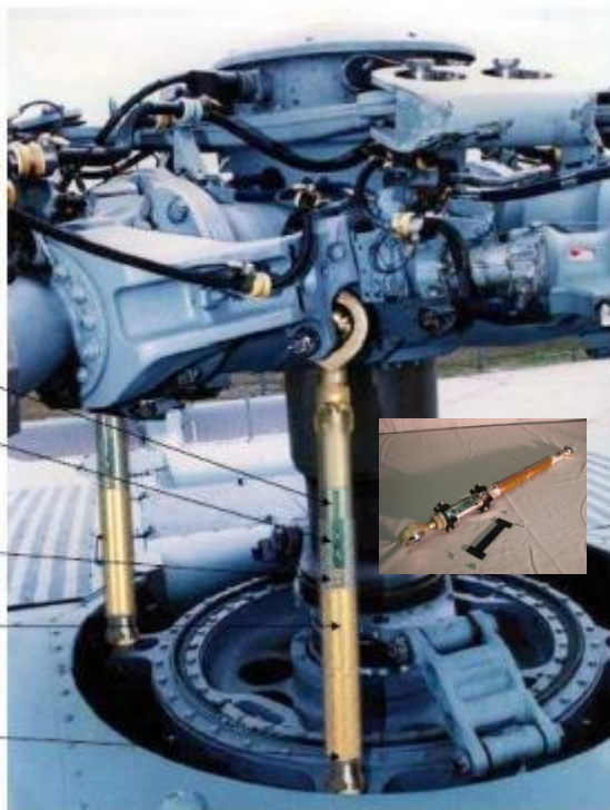
Helicopter Pitch Link w/ Energy Harvesting, Sensing, Data Storage, & Wireless Communications (MicroStrain, Inc. patents pending)
