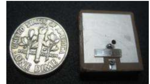
Miniature 915MHz Integrated OFC SAW-Patch Antenna
