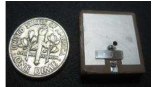
Miniature 915MHz Integrated OFC SAW-Patch Antenna
