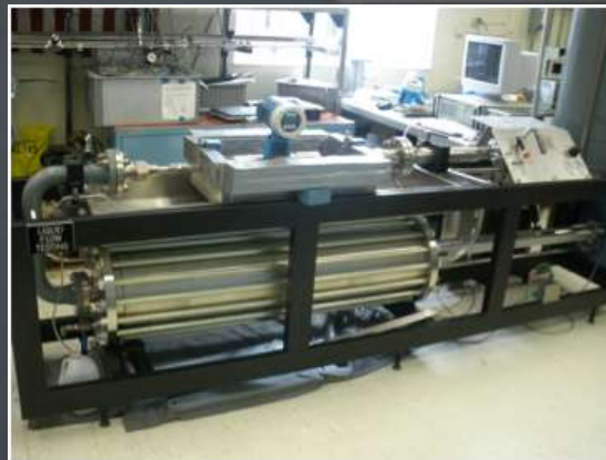
Piston Prover (flow meter testing)
