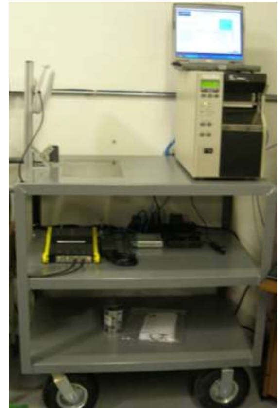
Commissioning cart holds antenna, reader, computer and tag printer.
