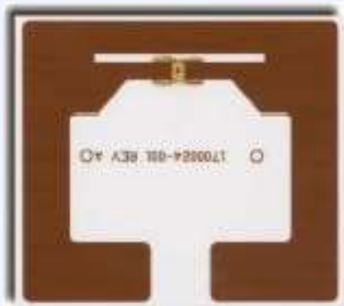
2"x2" Passive UHF (900 MHz) RFID Tag
