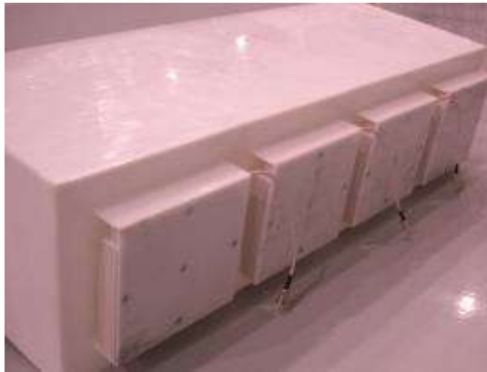
Freezer insert holds 4 antennas
