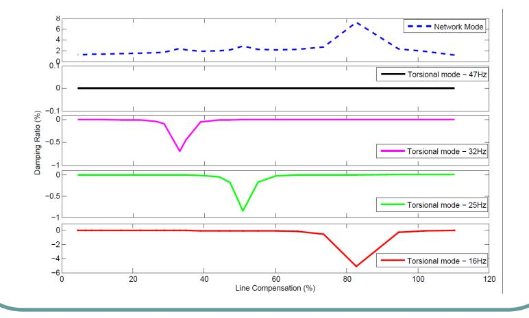
When Network mode is close to 16 Hz torsional mode.
