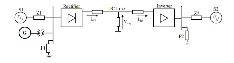
Torsional interactions occur when there is a lightly damped oscillatory mode in the HVDC system close to one of the torsional modes – weak resonance condition
