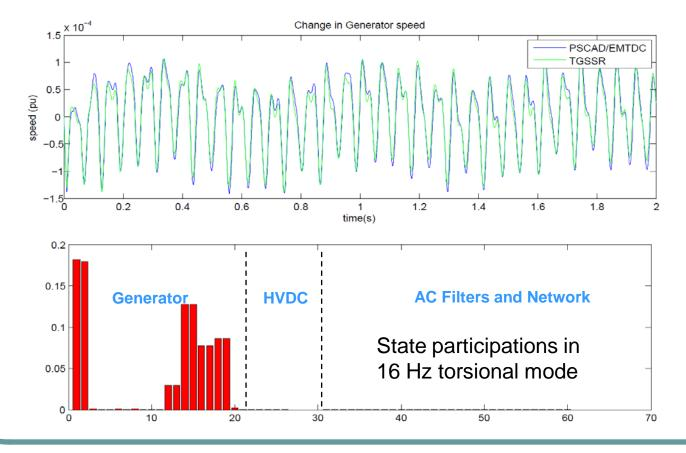
• Current controller gains were adjusted to create a oscillatory mode close to 16 Hz.
