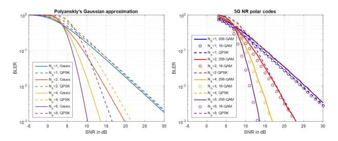
Block error rates for transmission of 192 info bits in 128 resource elements (R = 1.5 bit/use) over  $N_{\rm b}$  Rayleigh fading blocks. Theoretical results (left) and 5G polar codes (right).
