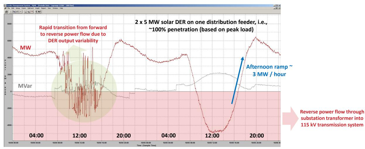
One-minute real & reactive power flow measured at substation bus, 48-hour period
