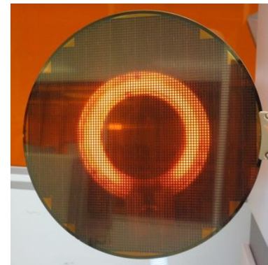
SM95 wafer in front of a lamp showing semitransparent membranes formed by DRIE
