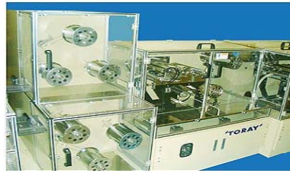
Coating and Exposure (resolution: L/S = 10/10 \mu\text{m} ) (Toray)
