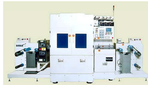
Coating and Exposure (resolution: L/S = 10/10 \mu\text{m} ) (Toray)
