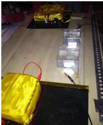
Power hop across structures and saltwater filled chambers.
