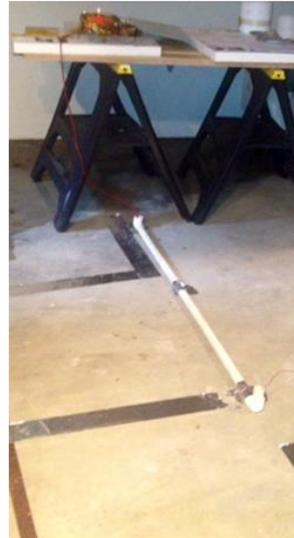
Power hop across metalized tape and saltwater filled PVC. Collective 10 meter separation
