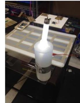
Direct Excitation of Plasma via Salt Water Conductive Plane
