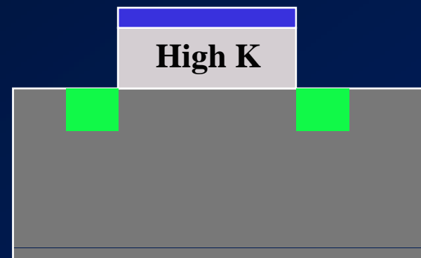
Transistor with high K gate oxide
