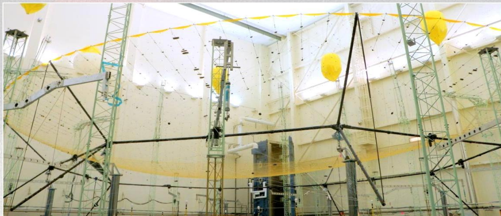
Harris 22 meter Antenna (Hoop Truss)
