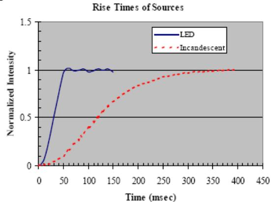
The faster rise time will alert drivers more quickly. The European Lamp Companies Federation reported that LEDs "illuminate 99% faster than incandescent car lamps resulting in a reduced stopping distance of 8 m at 100kph. Eight meters equals the length of up to 2 cars and can be the difference between life and death in a head-tail collision."
