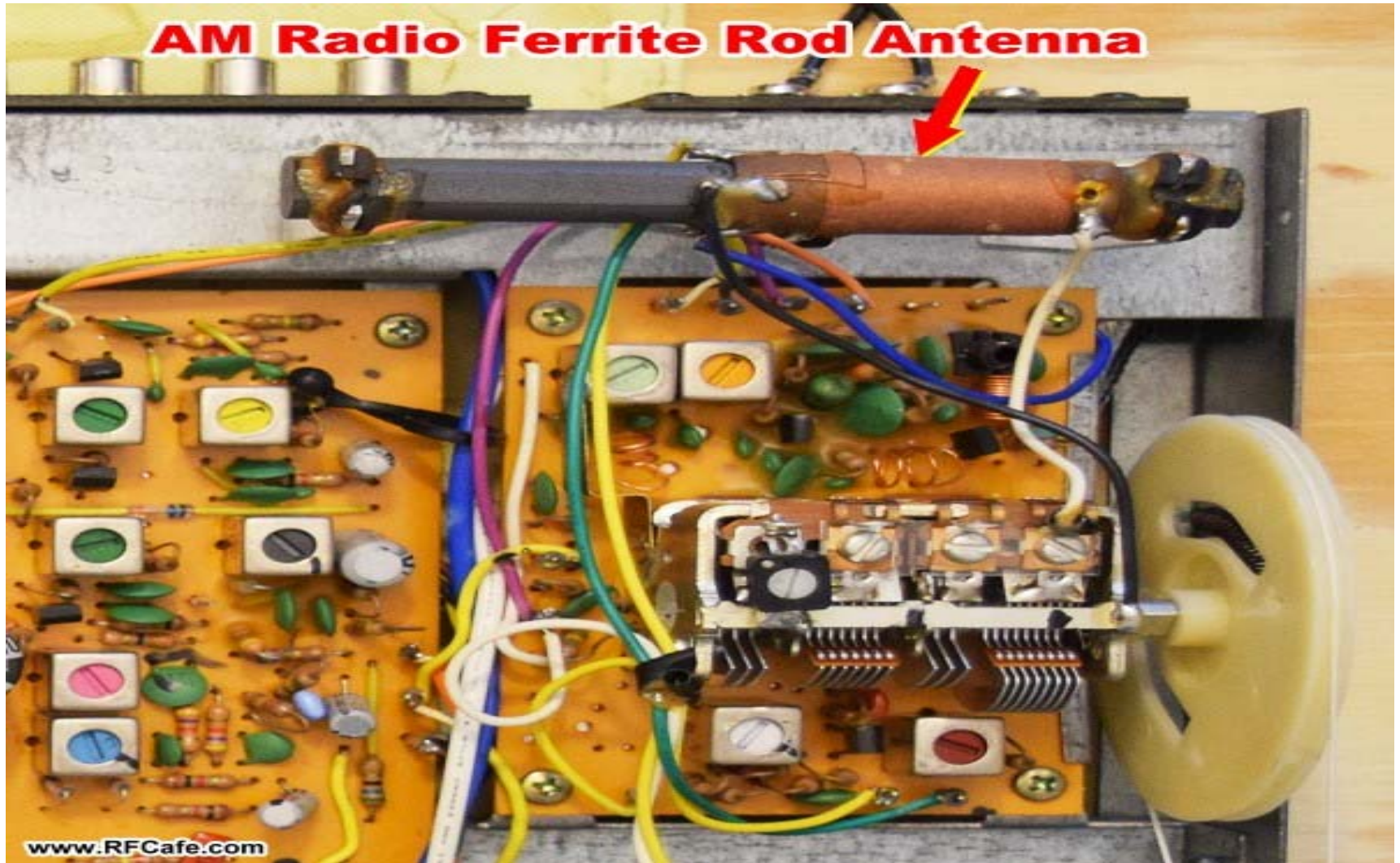
Antenna inside a prehistoric transistor radio
