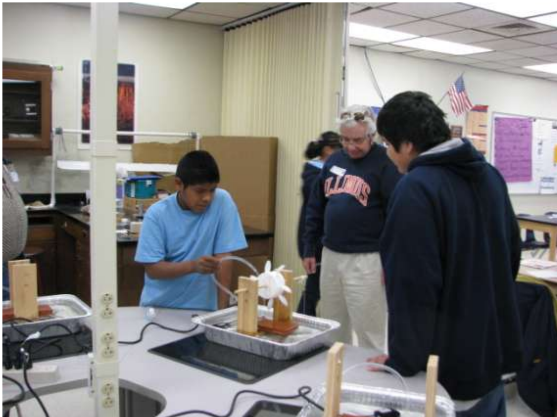
Many Students Initially Went For A Design Using Spoons As Paddles Until They Saw The Performance Advantage Colleagues Using Small Cups Had Over Them
