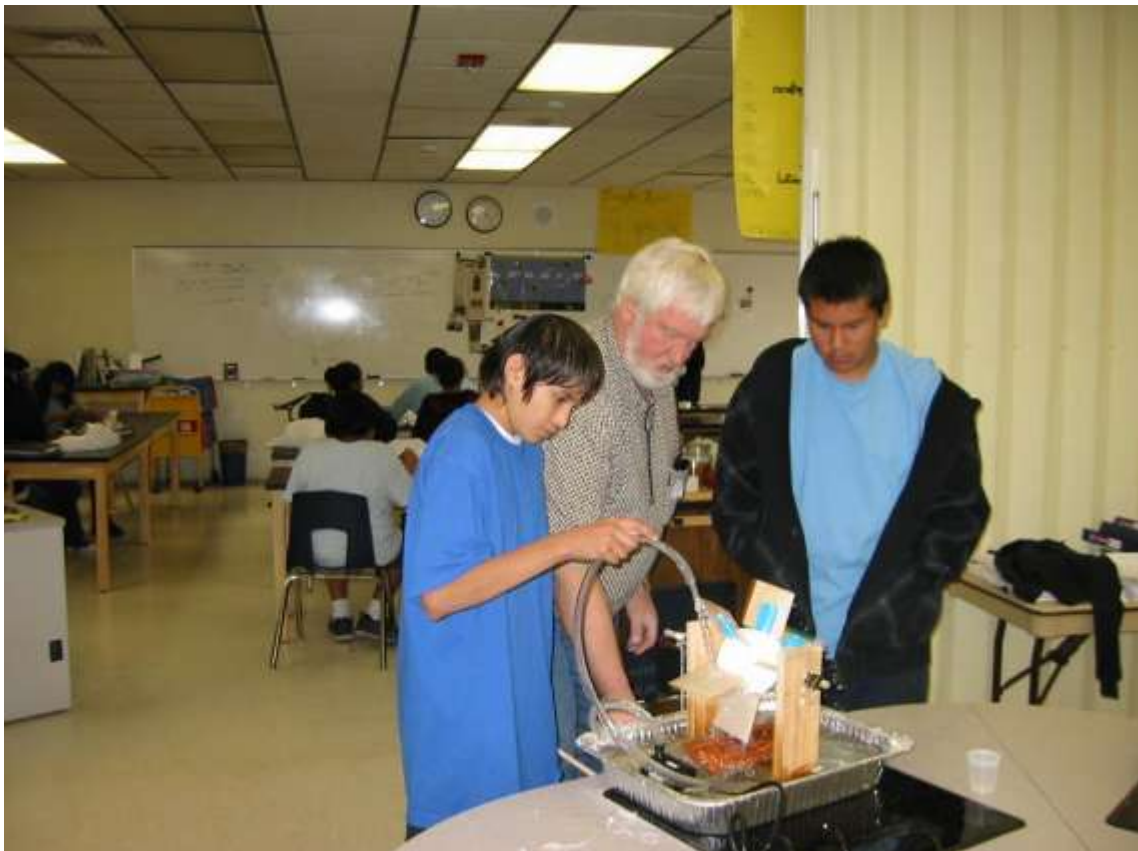
A Large Paddle Design — It Would Have Worked Better If We Had Had A Stronger Water Jet From The Fountain Pump We Were Using!
