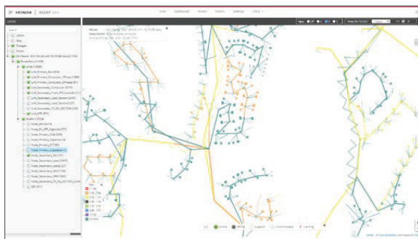
Feeder with voltage levels
