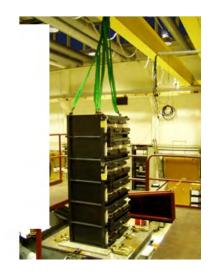
Of safety reasons the cells were filled with glycol when the rack was tested. The mechanical strength of the rack was then verified, but not the electric function of the cells.
