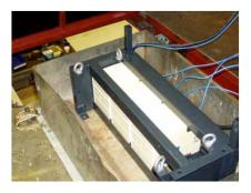
During the test of the rack, secondary spectra were measured at the rack and these spectra used at a test of with aged cells filled with acid (placed in a stainless tray). During this test the electric function was monitored.
