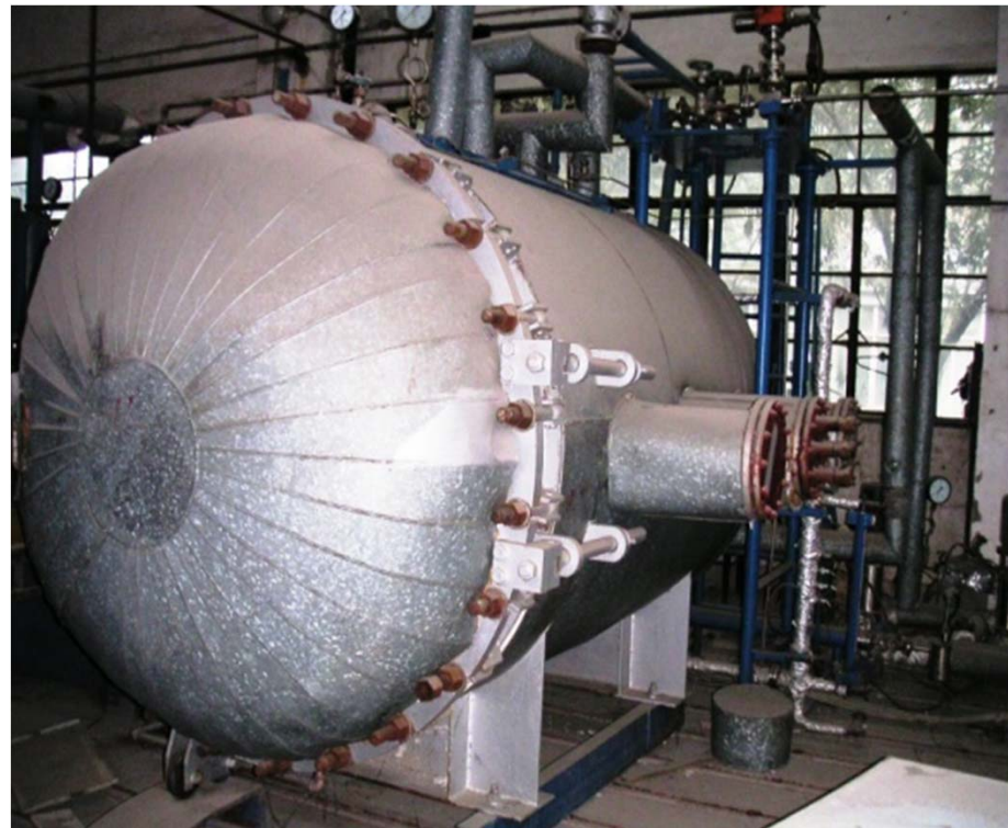
A LOCA Facility ever used for 300MWe design in SNERDI
