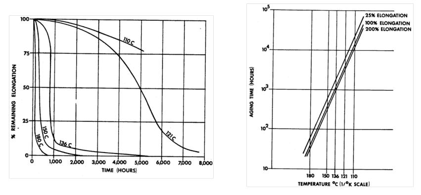
Arrhenius modeling of % elongation of jacket material complete at Draka (BIW) on Bostrad<sup>7E</sup> cables. The rate of aging determination allows a line to be extrapolated through the desired service condition.
