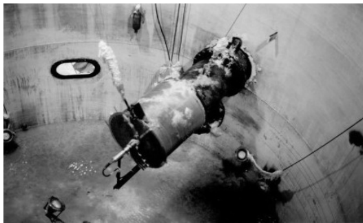
36" Prototype Active Strainer Test Performed at EPRI in 1995
