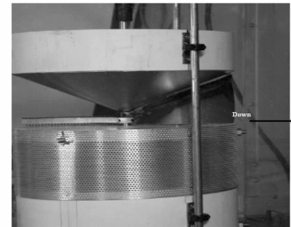
12" Prototype Active Strainer Used in Proof of Design Testing Performed in 2003
