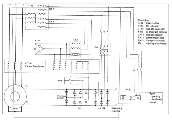
Devices T102, C101, L101, T101, A111, T103, A114 comprise the part of the new design called the "magnetics." These components produce rectified DC field current that is a function of DG no-load and load components capable of regulating DG output voltage to  $\pm 4.8$  percent.
