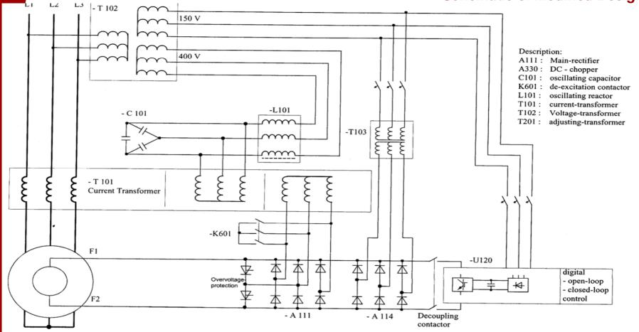
In event digital AVR (U120) malfunctions, an over/undervoltage relay disconnects the AVR by opening the decoupling contactor. Diesel generator continues to operate within Tech Spec voltage limits using the "magnetics" to supply field current but without ability to raise or lower voltage.
