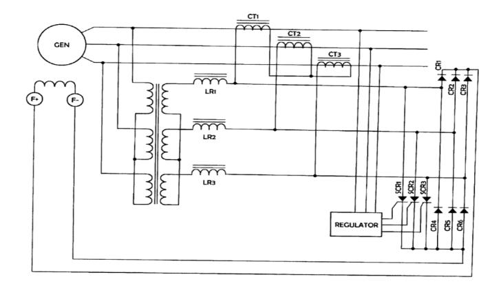
Existing excitation system consists of three, single phase power transformers, two three phase sensing transformers, one 800/5 reactive current transformer, three power current transformers, 3 linear reactors, one three phase power output rectifier bridge with shunting Thyristor (SCRs), normal and standby automatic voltage regulators, a remote gate firing module, power driven pot (PDP), relays and control switches. Most of these components are obsolete and spare parts are no longer available.
