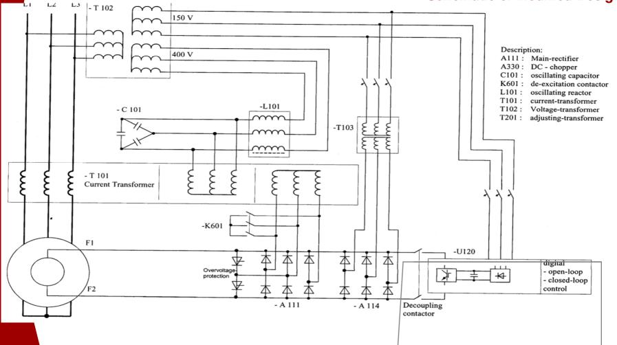
Device U120 at lower right is the digital AVR. This component produces rectified ±DC which boost (+) or bucks (-) output of "magnetics" allowing regulation of DG output voltage to ±0.5 percent, and allow raising and lowering of voltage for such functions as synchronizing to the grid.
