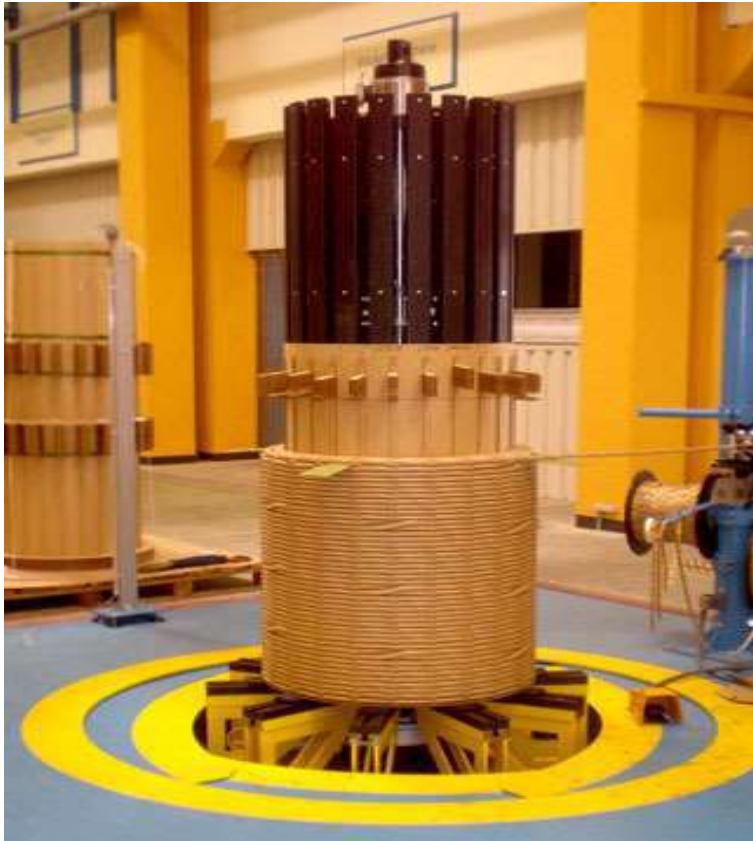
Old Vertical winding machine without breaking mechanism
