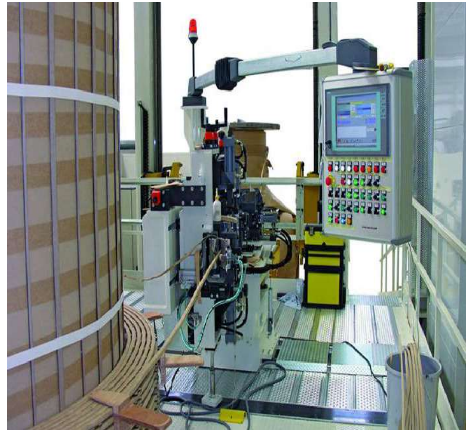
New Vertical winding machine with breaking and tension mechanism
