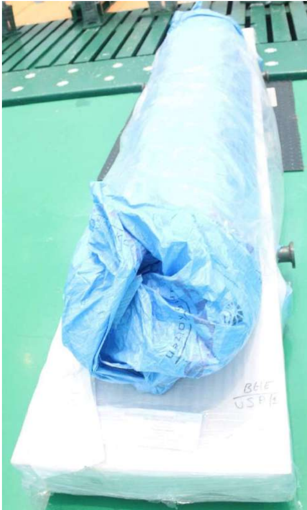
Core steel packed to prevent rust
