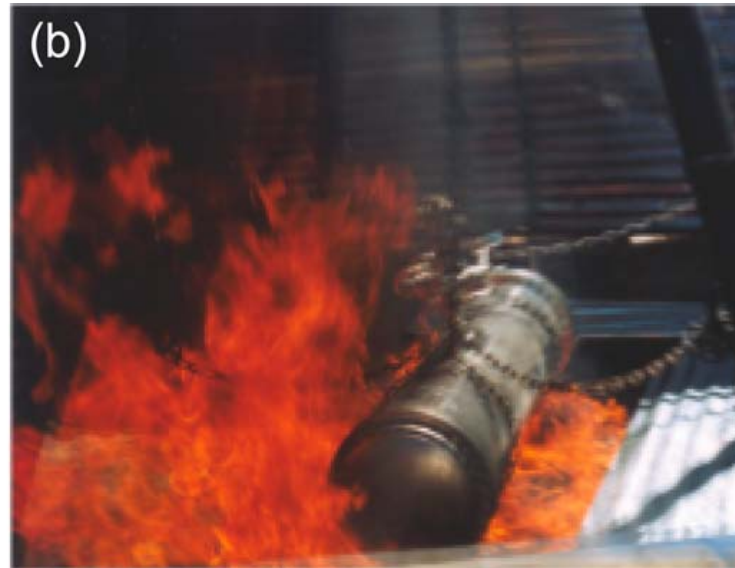
(b) bathing the tank in flames for over 60 minutes at 1000 C
