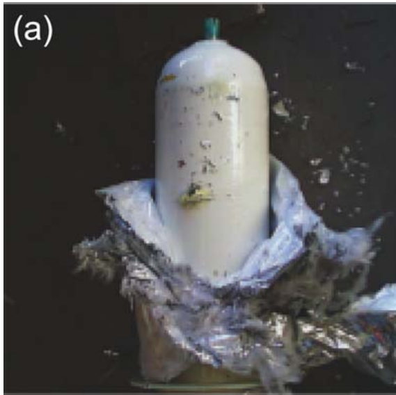
(a) piercing the tank with .30-caliber armor-piercing bullets
