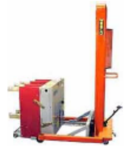
2. Roll Circuit Breaker on Truck Lift
