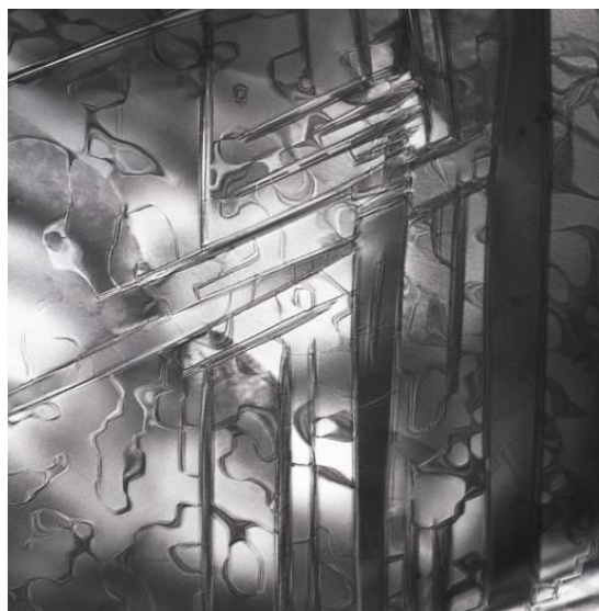
Figure 1. Bright field TEM image illustrating V_{\text{Sr}} and O tilt superstructure in rare earth doped \text{SrTiO}_3
