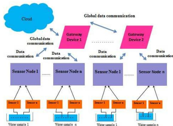
Figure 1: Fog Computing based System Framework
