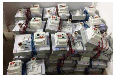
The students prepared 610 temporary electrical connection boards consisting of isolator, ELCB, a lamp holder, a 3-pin power socket and an LED indicator. These boards were used to connect electrical supply from KSEB's service main board avoiding the damaged wiring of the houses.
