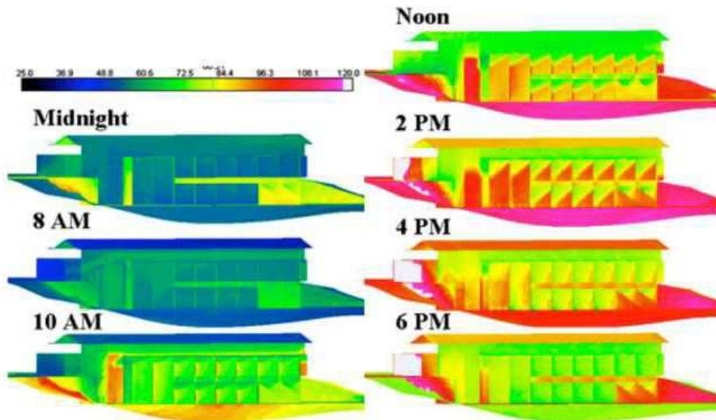
Figure 3: Energy analysis at different times during the course of a day
