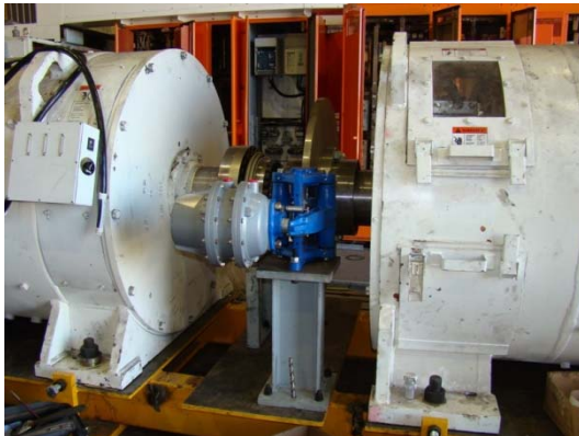
Figure 2. Hoist motors on a dynamometer test bed.
