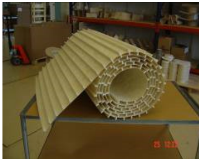
Duct Strips for oil flow
