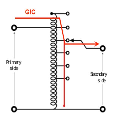
GIC flows from high side through series winding to low side, and through common winding to ground
