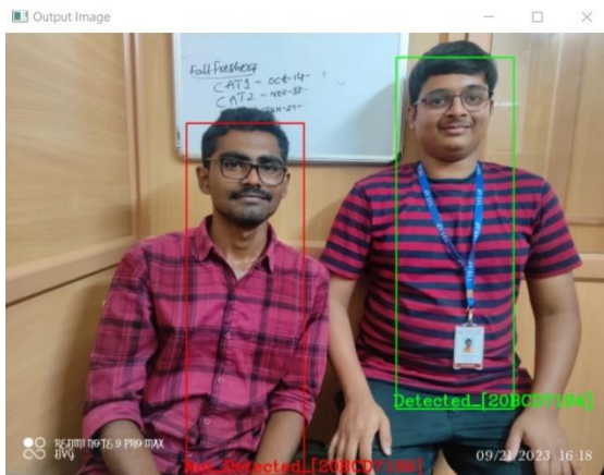
Figure 2. Output screenshot of Integrated Face and ID Card Image Detection System detected images using YOLOv8
