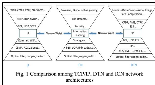
There are basically two effective standardized network architectures for space internetworking [1], i.e. TCP/IP (IP over CCSDS) and Delay-Tolerant Networking (DTN), as shown in Fig. 1. Designed for terrestrial networks,
