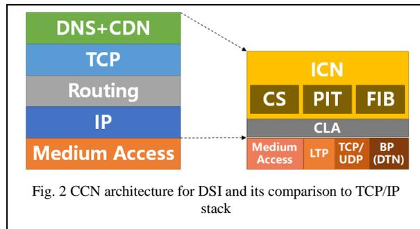
Fig. 2 CCN architecture for DSI and its comparison to TCP/IP stack
