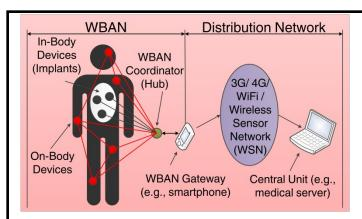
Figure 2. Wireless body area network: a macro network comprising many sub-networks involving on-body, in-body, and hub devices connected to a core network (i.e., server) using different radio access technologies.
