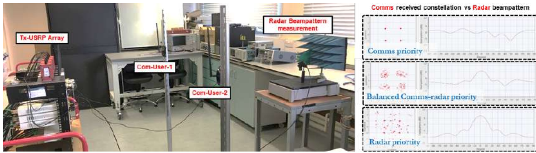
Figure 3.6: Proof of concept DFRC experiments in UCL. The communications-sensing trade-off over the air.
