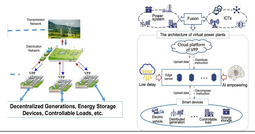
Virtual power plant (VPP) can aggregate the capacity of distributed resources through the fusion of power system and Information Communication Technologies
