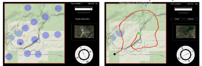
Fig. 3. Participants controlled the UAS using a stick-and-carrot control scheme (left panel): clicking the map would set a new destination for the UAS (red reticle). Once arriving at the destination, the UAS would orbit until retasked. Participants searched for targets located in half of the blue potential target locations on the map. After completing the task, participants attempted to reconstruct their route by drawing it on the map space (right panel).
