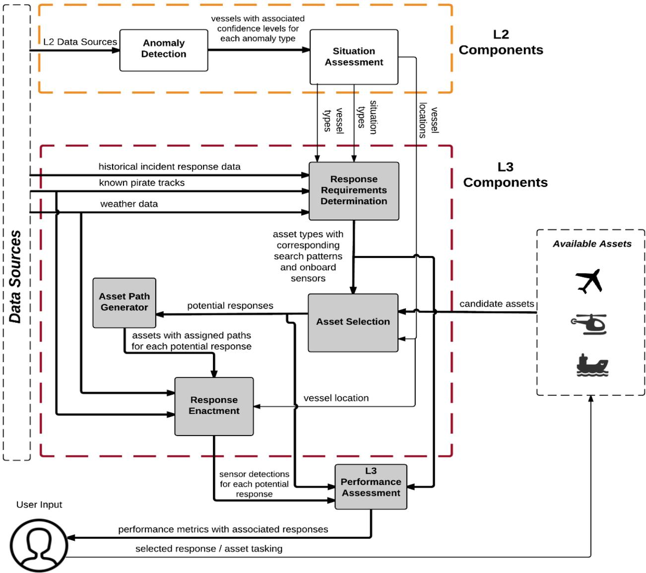
Fig. 4. Soft-Data-Driven Response Generation (SDDRG) System
