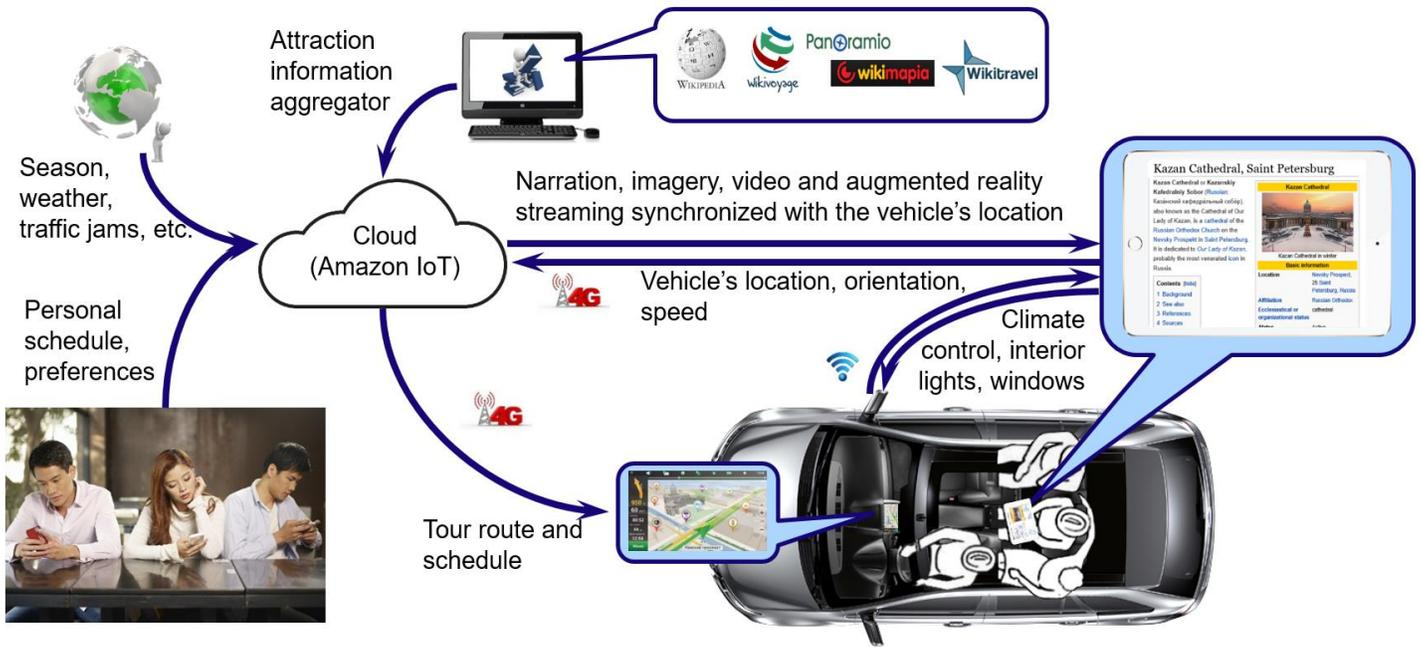
Fig. 3. Cyber-physical-human system for connected car-based e-tourism: case study
