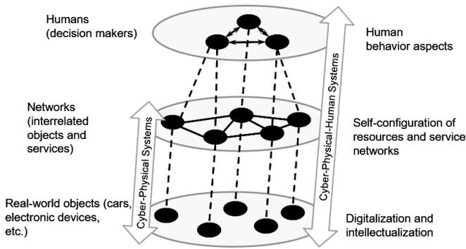
Fig. 1. Cyber-physical and cyber-physical-human systems
