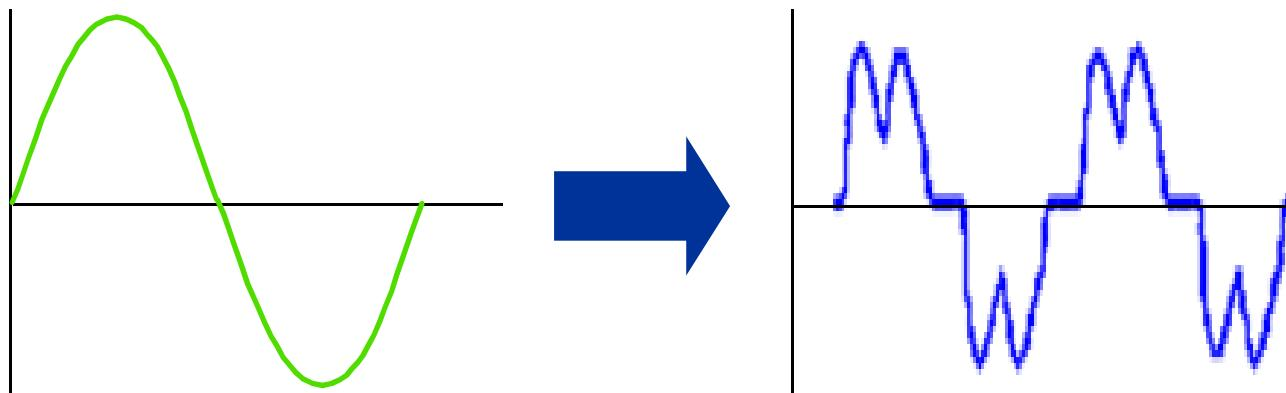
...but nonlinear devices distort voltage and current waveforms resulting in poor power quality on the distribution grid with further implications
