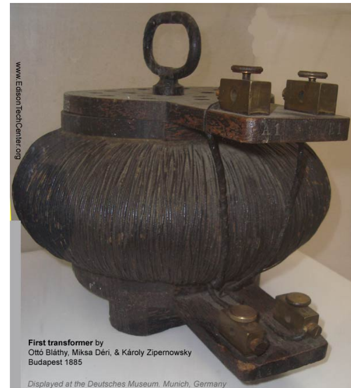
BDZ: 1885 toroid-core transformer
